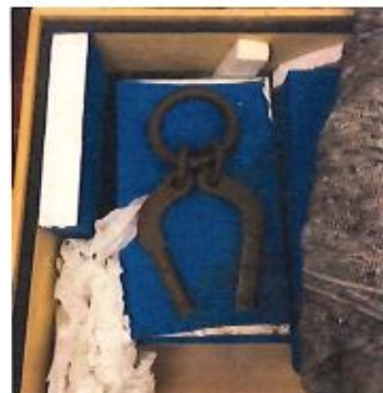
Split steel pin for moving artworks – the two loose sections need to be joined together to form a circle and inserted into the holes (see above images).
